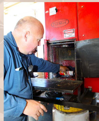
An employee places a can of spray paint into a machine that will safely remove remaining liquid and store it for disposal. Once processed, the can is ready to be recycled.
