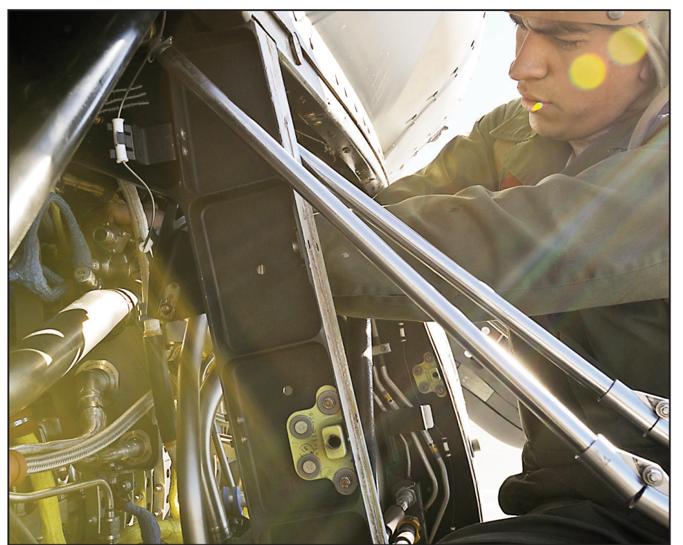
Cpl. Josue Alvarenga, Marine Medium Tiltrotor Squadron 363, replaces a cam plug on an MV-22 Osprey aircraft during Integrated Training Exercise 2-16 aboard the Combat Center, Jan. 24.
