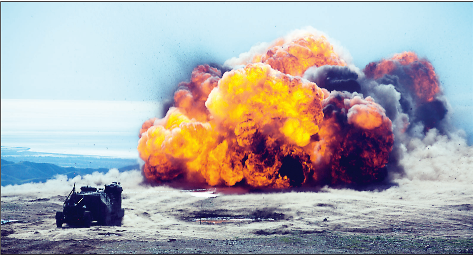
U.S. Marines and Japan Ground Self-Defense Force soldiers detonate a Mine Clearing Line Charge to clear an obstacle, during a breaching training event, aboard Marine Corps Base Camp Pendleton, Calif., Feb. 4. The MCLC contains 1,750 lbs of C4 explosives and is launched into a forward area by a rocket to clear a path.
