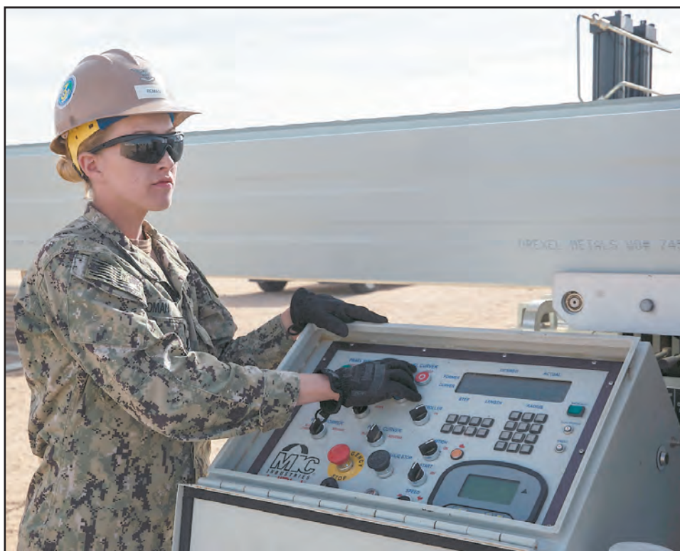
Petty Officer 3rd Class Laine Roman, main operator, Naval Mobile Construction Battalion 3, turns on the K-Span Machine to create the metal sheets used to create the K-Span units at Camp Wilson aboard the Marine Corps Air Ground Combat Center, Twentynine Palms, Calif., Feb. 2. NMCB 3 is in Camp Wilson for three weeks working on the construction of displacement walls and K-Span units for their upcoming deployment in April.
