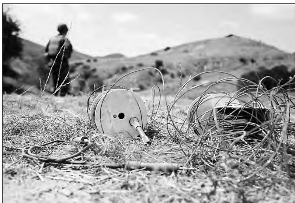
An In-Line Initiator M23 Blasting Cap Assembly lays on standby during a breaching and demolition training exercise at Camp Pendleton, Calif., Sept. 19. The M23 is used to propagate a detonation wave to a crimped and sealed blasting cap.
