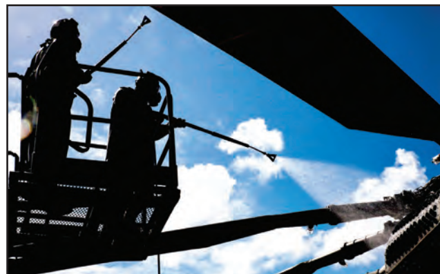
Marines with Marine Heavy Helicopter Squadron 463, also known as "Pegasus," Marine Aircraft Group 24, use a step ladder to power wash rotors from a CH-53E Super Stallion helicopter during a detailed aircraft decontamination exercise, aboard Marine Corps Base Hawaii, Nov. 8.
