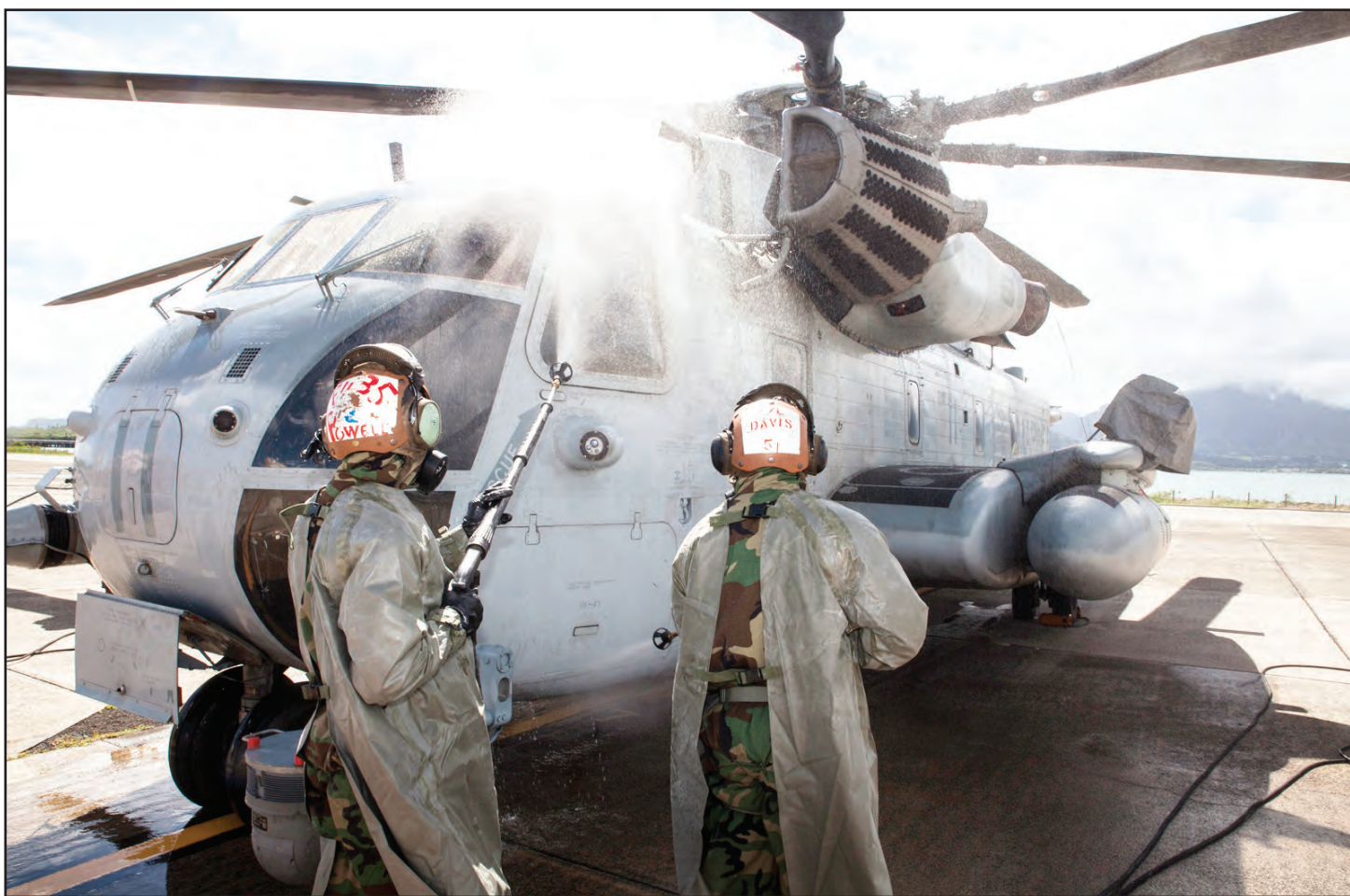
Marines with Marine Heavy Helicopter Squadron 463, also known as "Pegasus," Marine Aircraft Group 24, power spray a CH-53E Super Stallion helicopter during a detailed aircraft decontamination exercise, aboard Marine Corps Base Hawaii, Nov. 8. The DECON exercise instructed Marines on proper techniques and procedures with responding to a C chemical, biological, radiological or nuclear contamination on a static helicopter.
