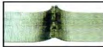
7. WEAR INDICATORS (RED CORE YARNS)
