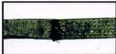
4. BROKEN OR WORN STITCHING
