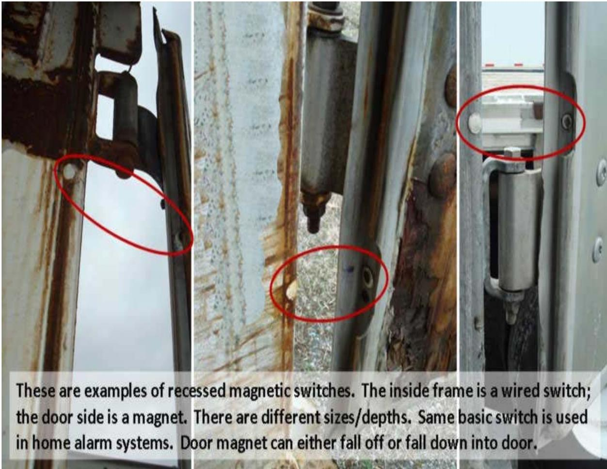
FIGURE 8-6. Trailer Tracking Door Contacts (Recessed)
