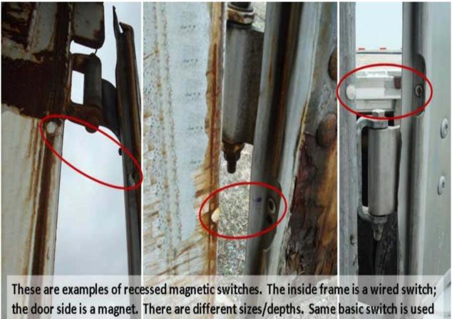
in home alarm systems. Door magnet can either fall off or fall down into door.
