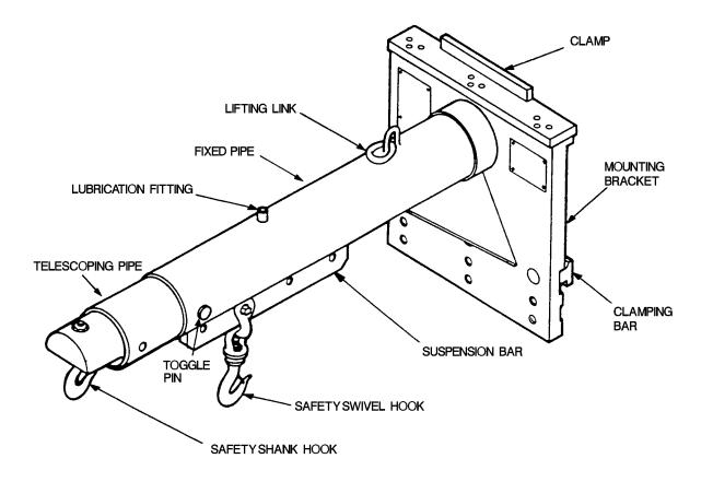
FIGURE 2-1. Mk 5 Mod 0 Forklift Truck Boom
