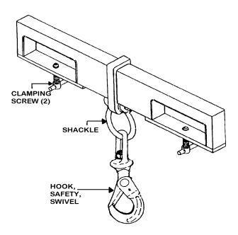
FIGURE 2-3. Mk 176 Mod 0 Hook Adapter
