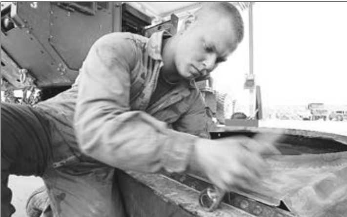
Cpl. Robert J. Lynn, a mechanic with Maintenance Company's Motor Transport Maintenance Platoon bolts a shroud onto a new radiator Saturday.
