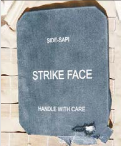
CPL. GRAHAM PAULSGROVE Ceramic small arms protective insert plates are designed to defeat multiple hits from assault rifles common on the current battlefield.
