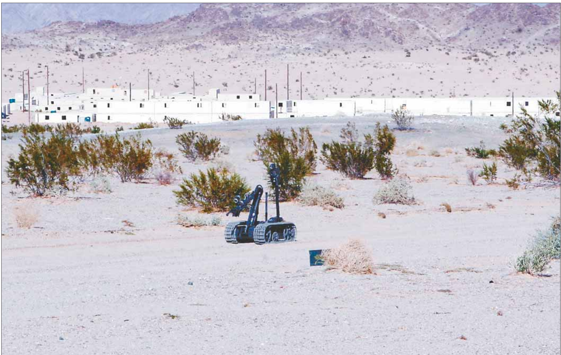
The Talon Robot is used by EOD Technicians to remotely investigate and neutralize suspected improvised explosive devices.
