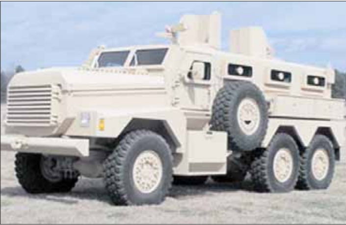
The 6 x 6 Armed Mine Protected Vehicle, dubbed the Cougar, is currently being used during combat operations in Iraq.
