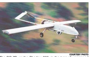
The RQ-7B, or the Shadow 200, is the type of unmanned aerial vehicle flown by VMU-3. The squadron will be activated at the Combat Center in September.
