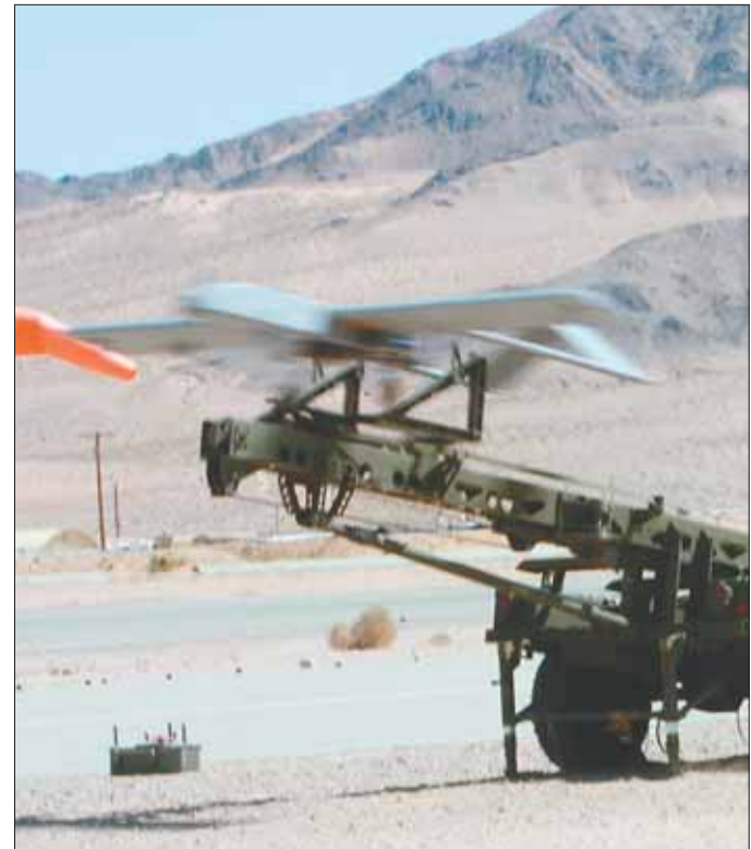
LANCE CPL. M. C. NERL The RQ-7B, known as the Shadow 200, shoots off the ramp as Staff Sgt. Jacksby Sewell and Sgt. James Marquardsen, both unmanned aerial vehicle operators with VMU-1, begin their qualification flight.
