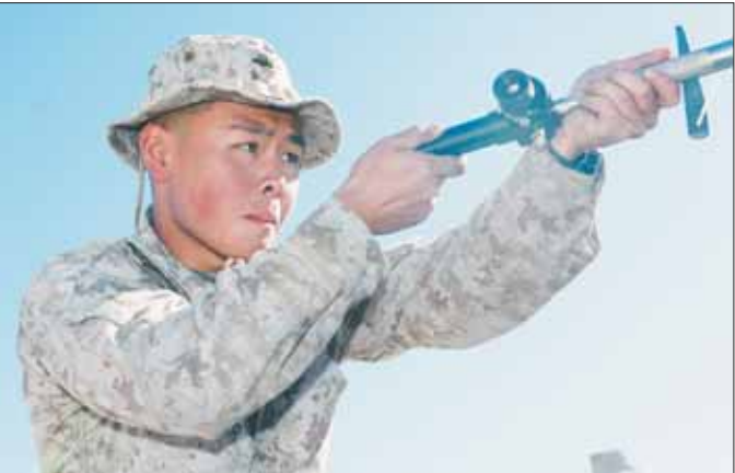
LANCE CPL. M. C. NERL Lance Cpl. Patrick Sharr, a light armored vehicle crewman with Company E, 3rd Light Armored Reconnaissance Battalion, aligns the bore sight on his 25 mm Bushmaster chain Gun Tuesday at the Combat Center's Range 109. The bushmaster is the main weapon on the LAV-25.
