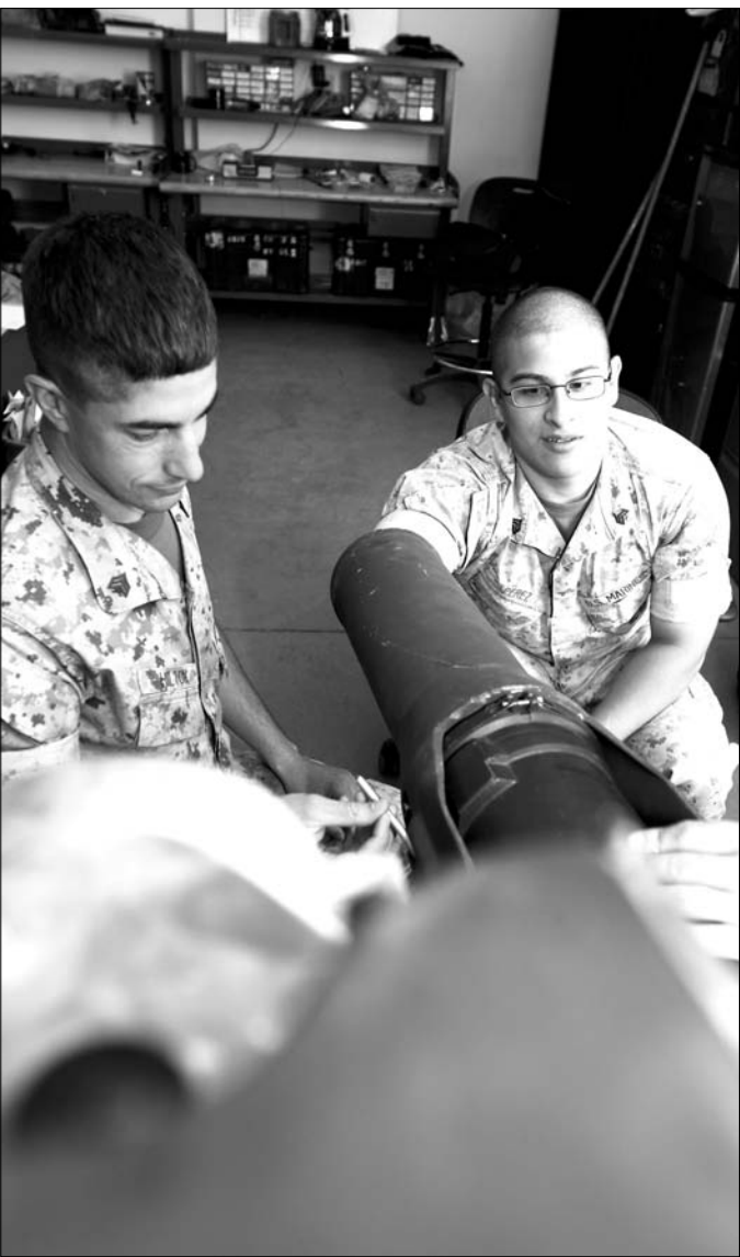
Sgts. Michael Hilton [left] and Phillip Perez, electra-optics repair technicians with 3rd Light Armored Reconnaissance Battalion inspect a Tube-launched, Optically-tracked, Wire-guided missile system Wednesday at the battalion’s optics shop. The shop handles repair on all sight systems and optical gear in the unit.
