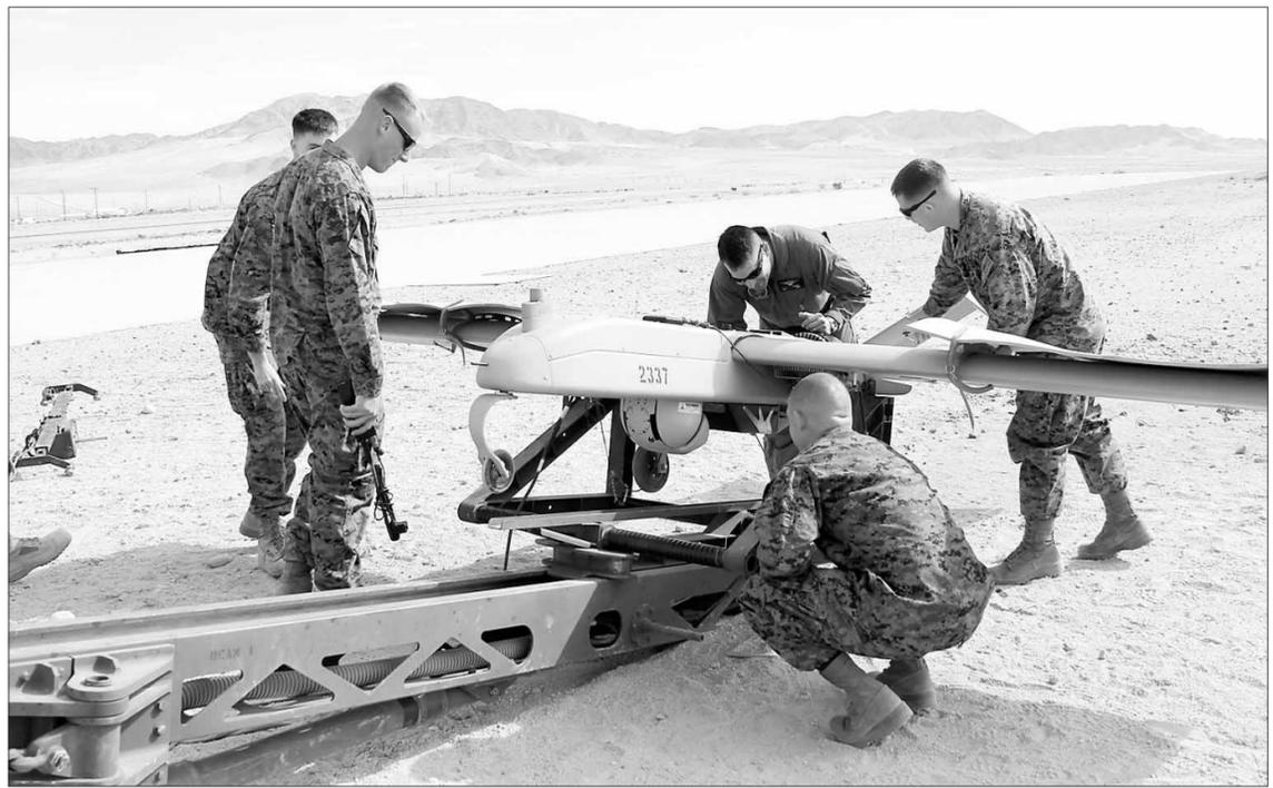
Vehicle operators and maintainers inspect an RQ-7B Shadow, unmanned aerial vehicle before launch at the Marine Unmanned Aerial Vehicle Squadron 1 airfield aboard the Combat Center Tuesday.
