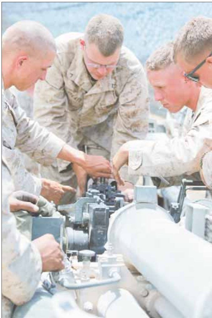
Marines with 2nd Battalion, 10th Marine Regiment, take apart the inside of the M777 A2 Howitzer to clean after firing. The excalibur round is rarely shot in training because of its $100,000 price tag.
