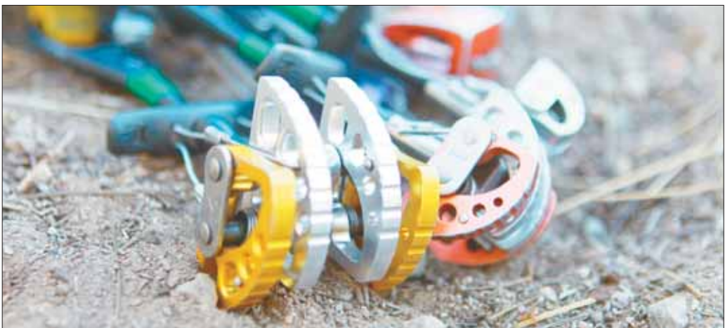
Spring-loaded camming devices, pictured above, are some of the many tools climbers use while negotiating rock faces. A cam is used by compressing a trigger, then inserting the cam into a crack or pocket in the rock. Releasing the trigger expands the cam. The friction between the cam and the rock is great enough that, when placed properly, it will hold the climber’s weight.
