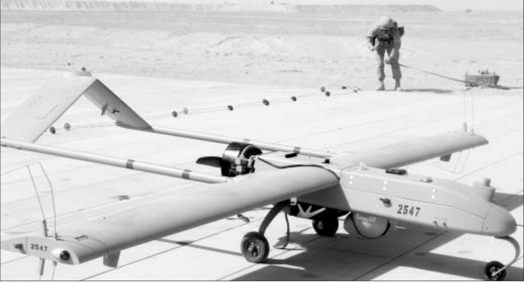
An RQ-7B Shadow is an unmanned aerial vehicle operated by VMU-3 in the skies of southwestern Afghanistan. Each Shadow carries a camera, which surveys and streams video to higher headquarters and ground units, giving them a full, accurate perspective of the battlefield.
