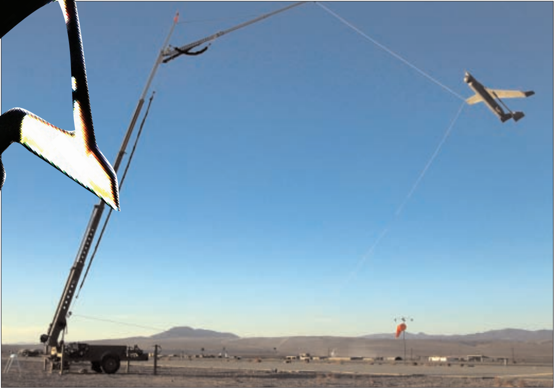
A new unmanned aerial vehicle, the Integrator, is recovered using a mobile catcher wire instead of the traditional landing strip a sneak preview for Unmanned Aerial Vehicle Squadrons 2 and 3 at the VMU-3 airfield Jan. 22.
