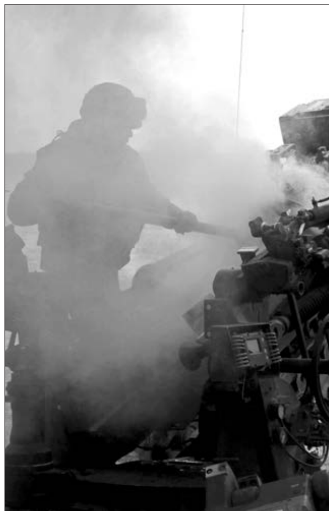
Marines serving with India Battery, 3rd Battalion, 11th Marine Regiment, swab the breach of an M777 Lightweight Howitzer after firing a round during a regimental exercise here Sept. 13. The exercise aimed to develop and sustain 11th Marine Regiment's ability to plan and execute artillery fires.
