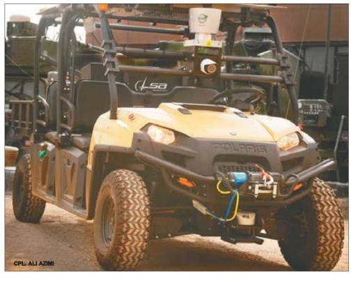
The Mobile Detection Assessment Response System uses color and infrared cameras, allowing operators to see things that Marines conducting ground patrols cannot. The system also utilizes a radar system to detect enemy presence and alert the operator.
