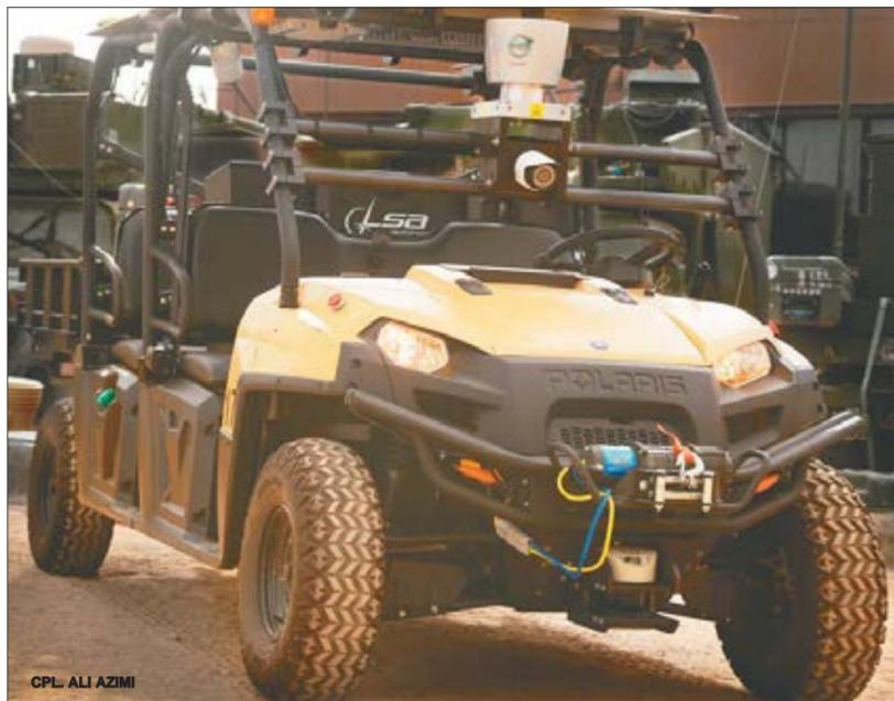
The Mobile Detection Assessment Response System uses color and infrared cameras, allowing operators to see things that Marines conducting ground patrols cannot. The system also utilizes a radar system to detect enemy presence and alert the operator.
