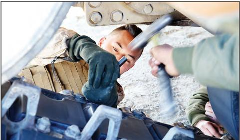
Cpl. Nick A. Buenviaje, tank gunner with Tank Platoon, Company B, Ground Combat Element Integrated Task Force, chisels debris out of the track pads to tighten the bolt during vehicle maintenance at Range SR-10, Marine Corps Base Camp Lejeune, N.C., Jan. 9.
