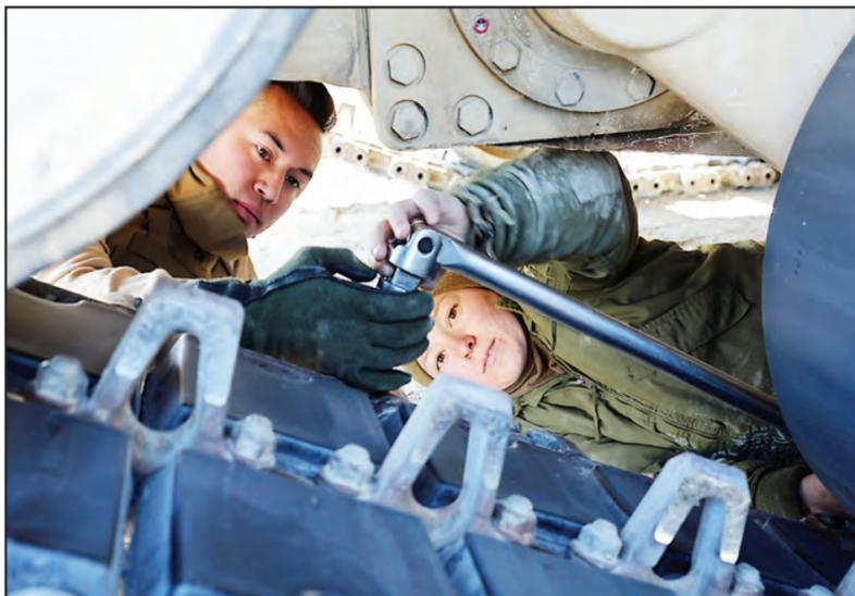
Cpl. Nick A. Buenviaje, left, tank gunner, and Sgt. Michelle A. Svec, tank crewman, both with Tank Platoon, Company B, Ground Combat Element Integrated Task Force, tighten a bolt on the track pad of an M1A1 Abrams tank during vehicle maintenance at Range SR-10, Marine Corps Base Camp Lejeune, N.C., Jan. 9.
