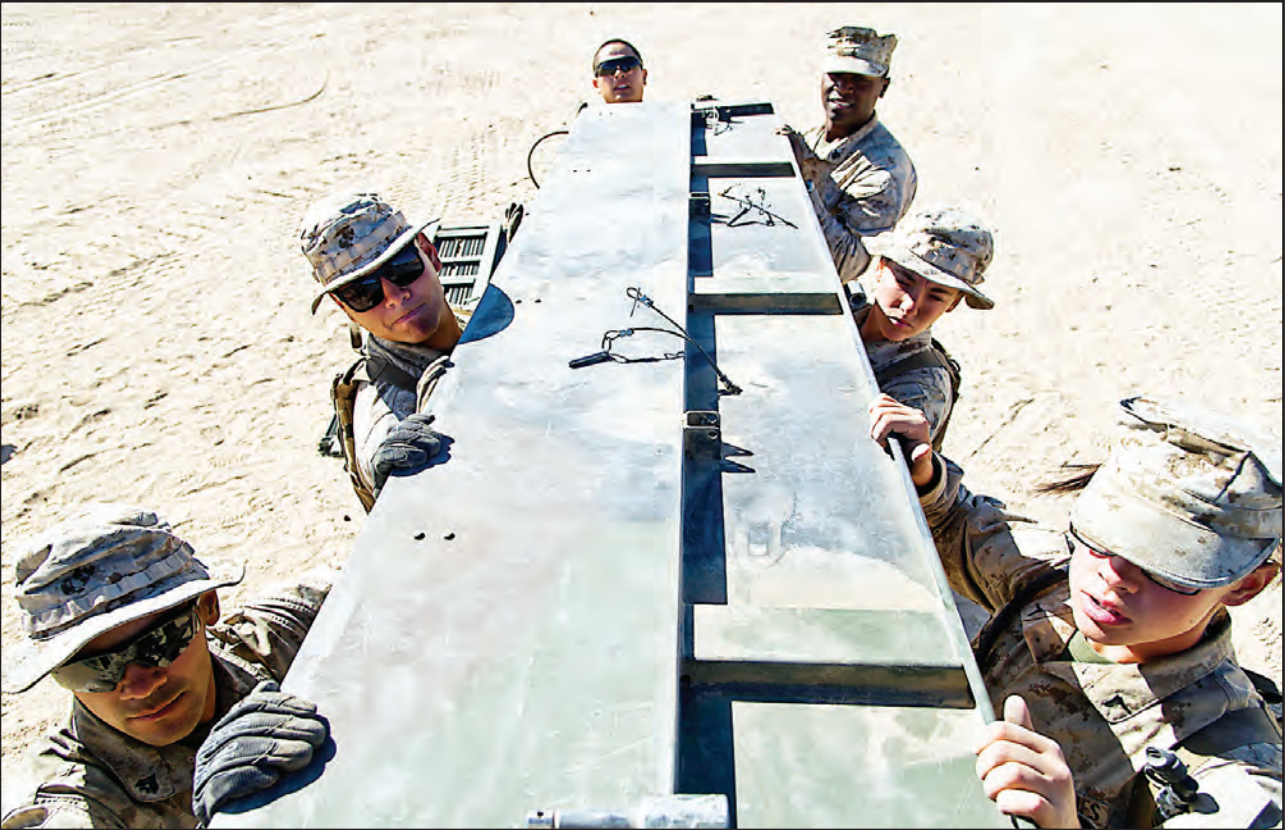
Marines from 1st Transportation Support Battalion, 1st Marine Logistics Group, remove the side rail and troop seats from a MK27 cargo truck during Integrated Training Exercise 2-15 aboard the Combat Center, Feb. 11.
