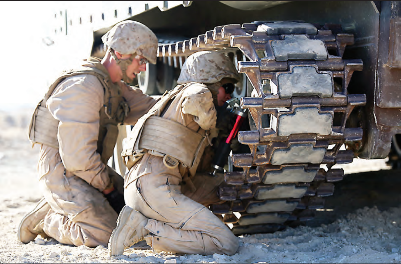
Sgt. Michael Meyer, left, crew chief, and Cpl. Kathryn Bynum, rear crewman, both with Amphibious Assault Vehicle Platoon, Company B, Ground Combat Element Integrated Task Force, work together to break track on an AAV during the assessment at Range 500, March 5.
