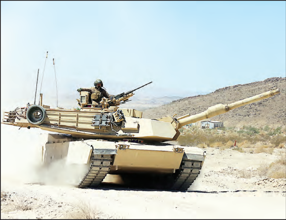
An M1A1 Abrams Main Battle Tank crew with Company A, 4th Tank Battalion, advances to its firing position during the company's pre-qualification tank gunnery at Range 500, Tuesday. The tank weighs approximately 70 tons and is capable of reaching a top speed of 45 mph.
