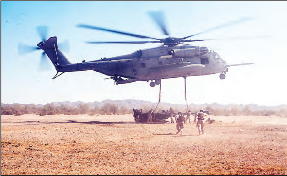
U.S. Marines with 1st Battalion, 10th Marine Regiment, 2nd Marine Division prepare to attach a M77 towed 155mm howitzer to a CH-53E Super Stallion during a CH-53 day battle drill in support of Weapons and Tactics Instructors course (WTI) 2-17 at Firebase Burt, Calif., Saturday.
