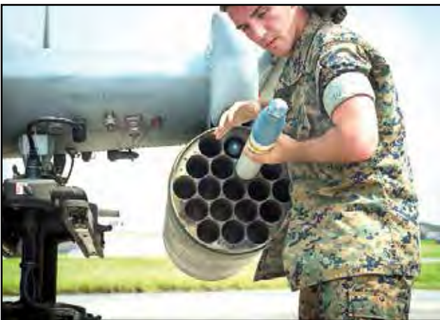
A U.S. Marine Corps ordnance technician with Marine Light Attack Helicopter Squadron 169 inserts a training missile into an AH-1Z Viper at Kadena Air Force Base, Okinawa, Japan, Thursday.
