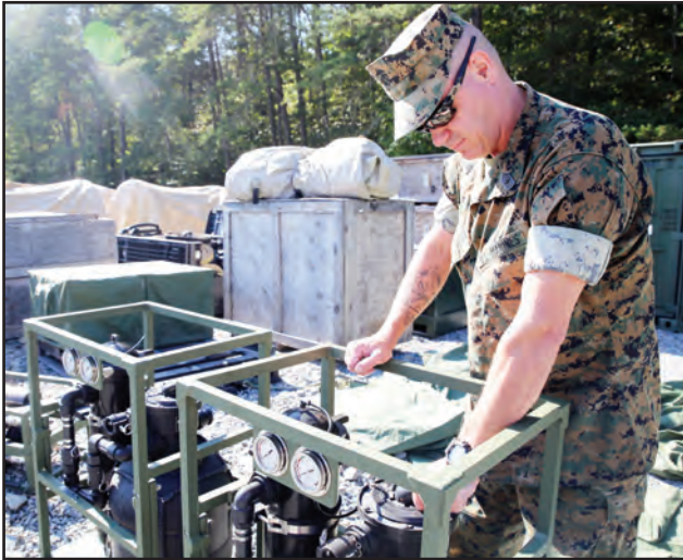
Master Sgt. Ryan Miller, project officer for Family of Water Systems at Marine Corps Systems Command, assembles the Lightweight Water Purification System with the new Enhanced Production Module. The EPM extends LWPS capabilities to an 80 percent increase in output and produces water faster for Marines.
