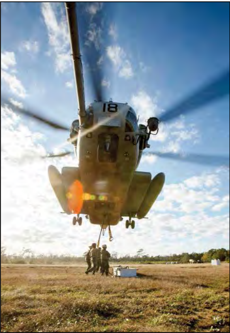
Marines with Combat Logistics Battalion 6, 2nd Marine Logistics Group attach cables and practice materials to a CH-53E Super Stallion during Helicopter Support Team training at Camp Lejeune, N.C., Tuesday. A Helicopter Support Team is comprised of approximately eight landing support specialist Marines who ensure the equipment is properly attached and secured before pilots transport the gear or supplies to their destination.
