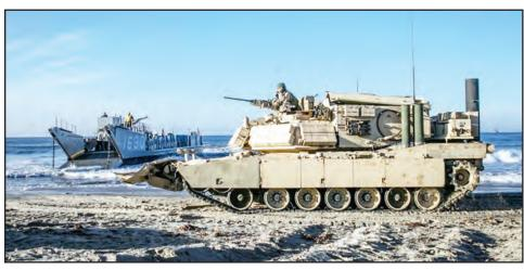
Marines from 1st Combat Engineer Battalion, 1st Marine Division, prepare to load an Assault Breacher Vehicle onto a Landing Craft Utility aboard Marine Corps Base Camp Pendleton, Calif. All vehicles were loaded onto LCUs then transported to the USS Rushmore to conduct the first amphibious landing in an ABV with a Modified Full Width Mine Plow prototype.
