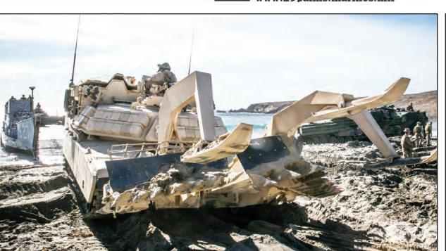
Marines from 1st Combat Engineer Battalion, 1st Marine Division, conduct the first amphibious landing in an Assault Breacher Vehicle with a Modified Full Width Mine Plow prototype during Exercise Steel Knight on the West Coast. Marine Corps Systems Command tested the prototype which will make it easier to transport the ABV from ship to shore.
